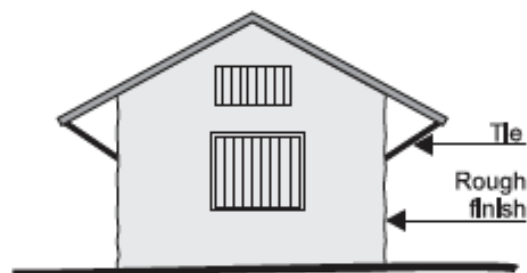
Sketch 9: Tie roof overhang @ 500 mm to wall
